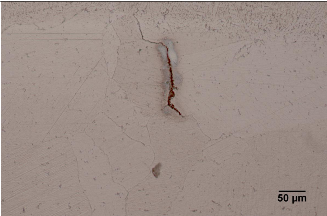
Figure 6. Optical Microscopy of liquation cracking in 700W LD Parent Material before heat treatment above, and post heat treatment below. (Author's work)
