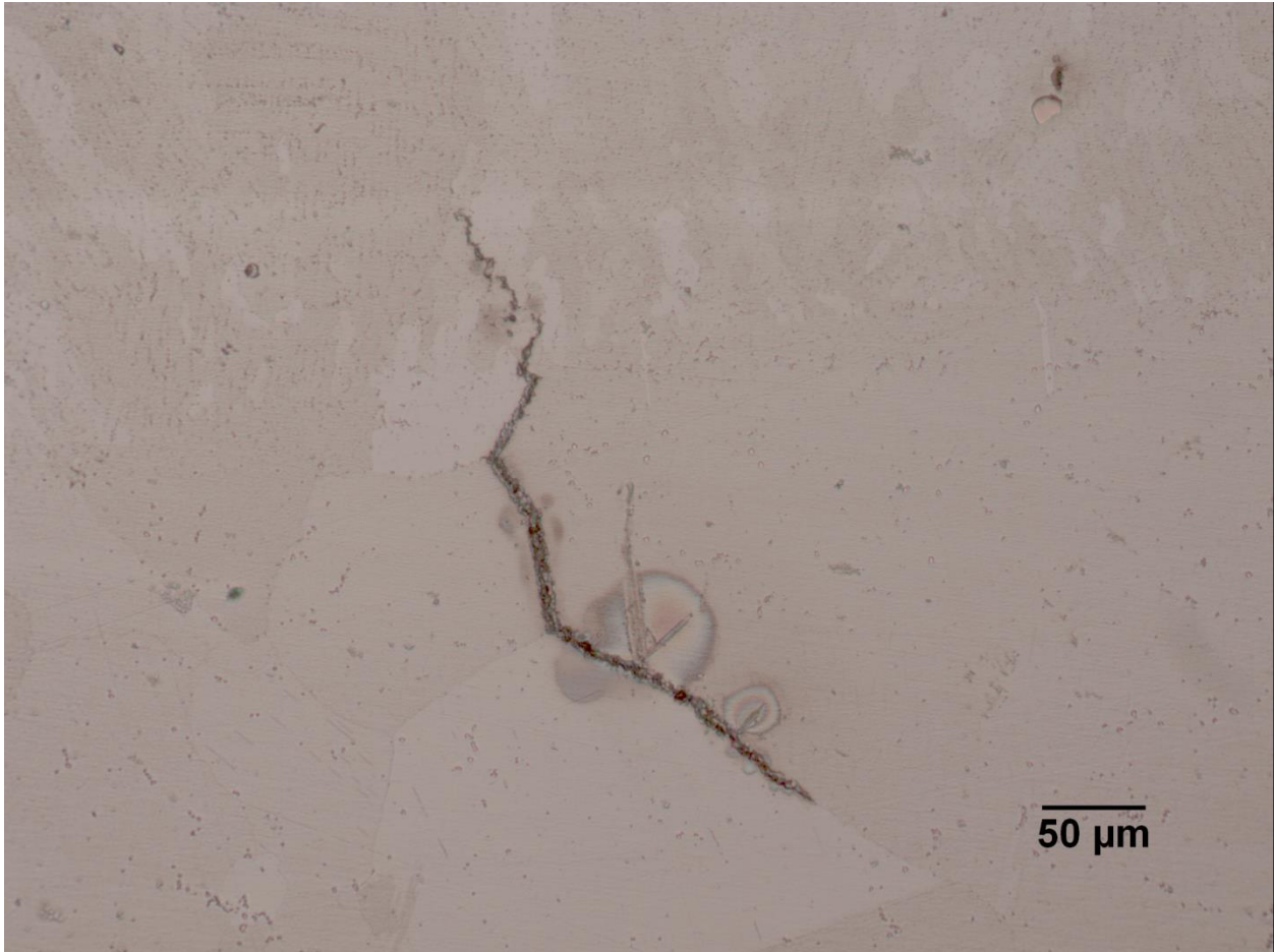
Figure 13. Micrograph of liquation cracking on 718 parent material with 900W Laser Deposition in post weld heat treated condition. (Author's Work)
